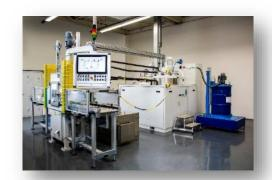
Specific drying and pre-heating of the components at device-specific temperatures and time-lines before encapsulation
